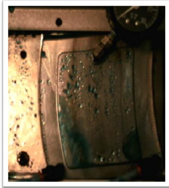
Figure 18 - Experimental Test with Clear Guide pads, Orifices on the Land at the Two Lower corners with no Channel into the pocket
