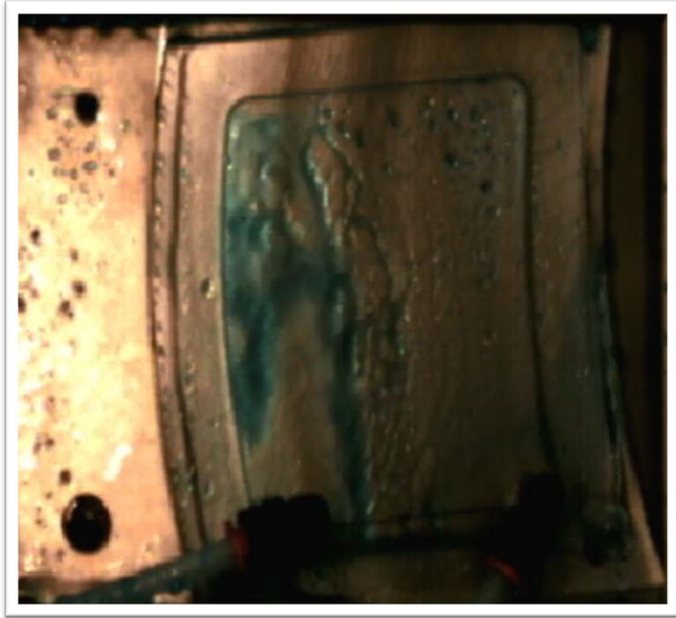
Figure 20 - Experimental Test with Clear Guide pads, Two Orifices inside the Pocket
